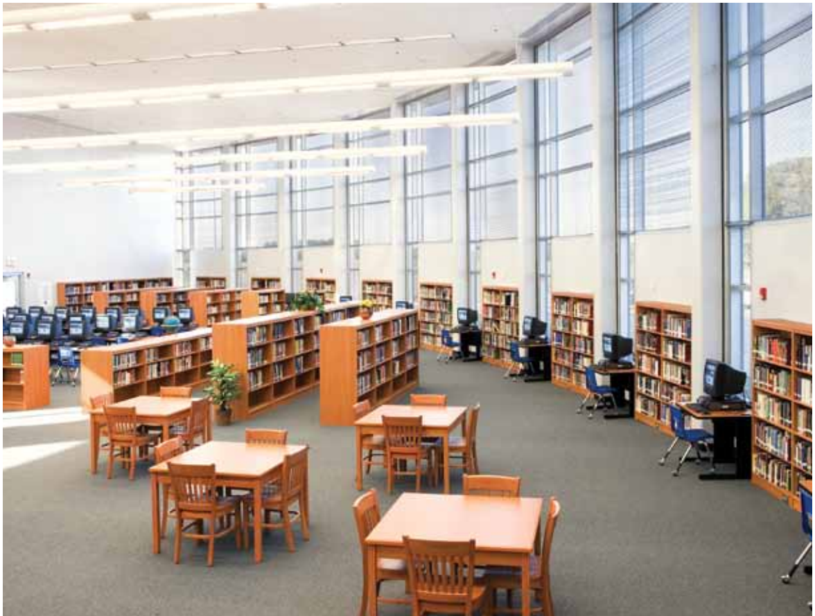
Figure 3 The insulated sandwich wall panels of the high school media center allowed the interior finish to be exposed painted precast concrete..
