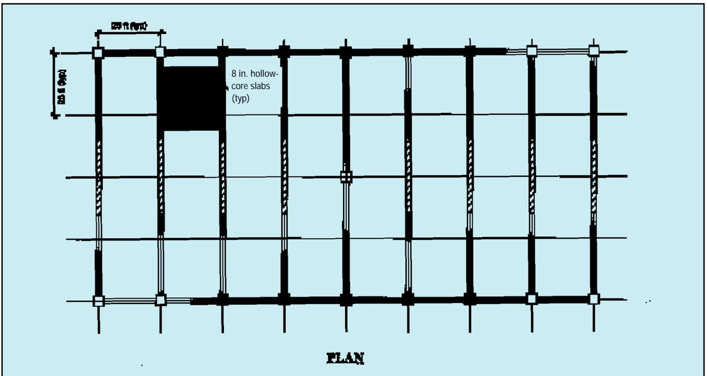
Fig. 2. Prototype building with topped hollow-core slabs. Note: 1 ft = 0.3048 m; 1 in. = 25.4 mm.
