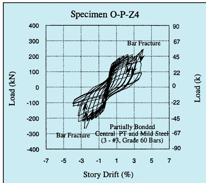
Fig. 9. Hybrid frame hysteresis loop (from Ref. 6).
