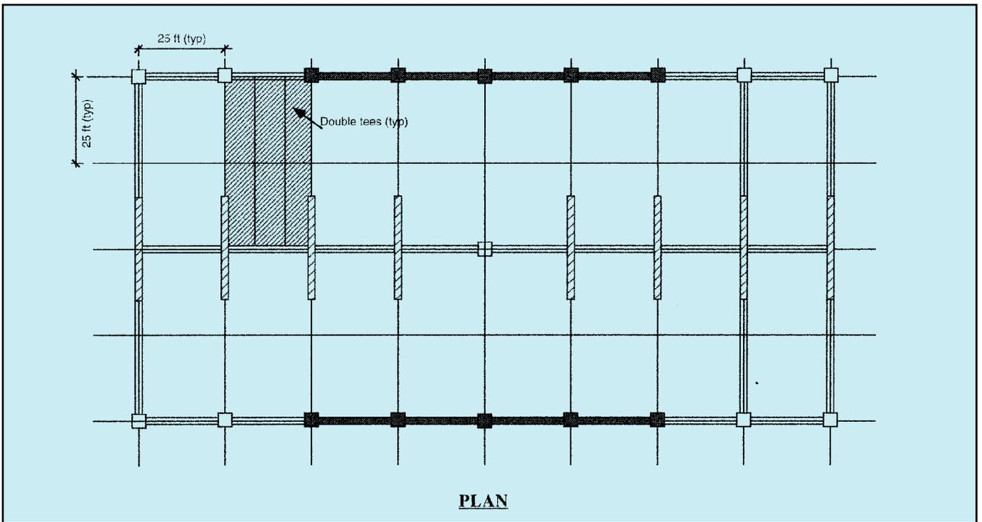
Fig. 1. Prototype building with pretopped double tees. Note: 1 ft = 0.3048 m.
