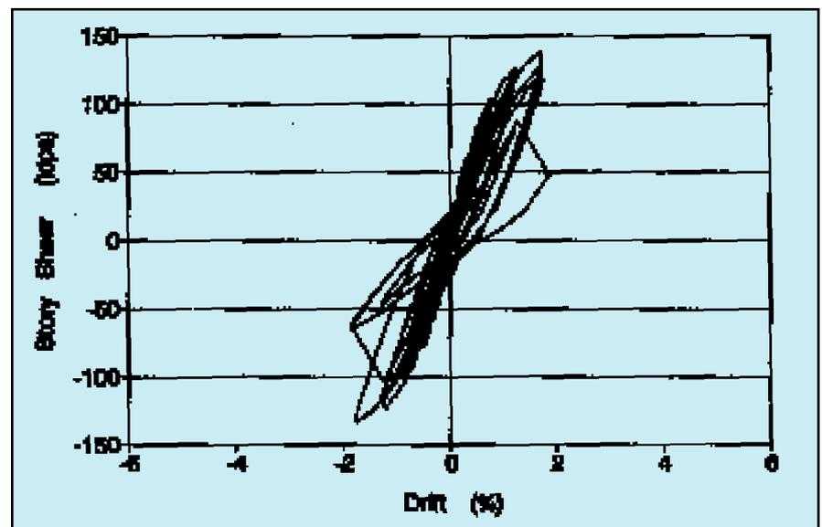
Fig. 13. TCY gap frame hysteresis loop (from Ref. 7).
