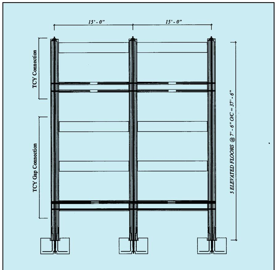
Fig. 7. Tension-Compression Yielding (TCY) frame elevation. Note: 1 ft = 0.3048 m; 1 in. = 25.4 mm.
