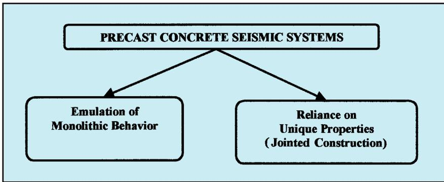
Fig. 3. Current code design choices for precast systems.
