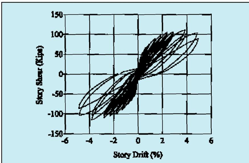
Fig. 11. Pretensioned frame hysteresis loop (from Ref. 7).
