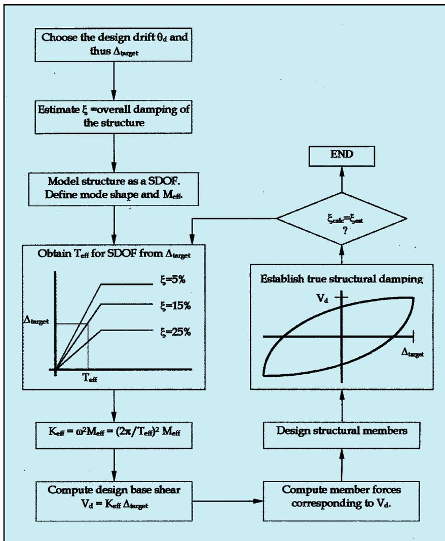
Fig. 18. Flowchart showing Direct-Displacement Based Design method.
